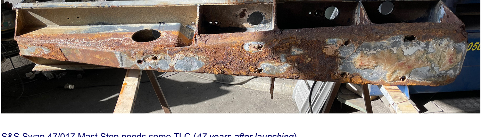
S&S Swan 47/017 Mast Step needs some TLC (47 years after launching)
